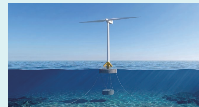
DDS-type floating offshore wind power generation Participating organizations: Kumagai Gumi Co., Ltd., Saga University, Yokohama National University, and CHODAI CO., LTD.
