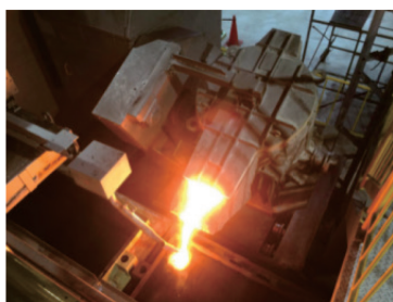
Photo.2 継手鋳造状況
