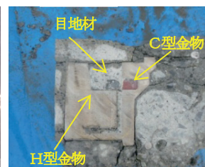
Photo. 6 切断観察 (充填性確認)
